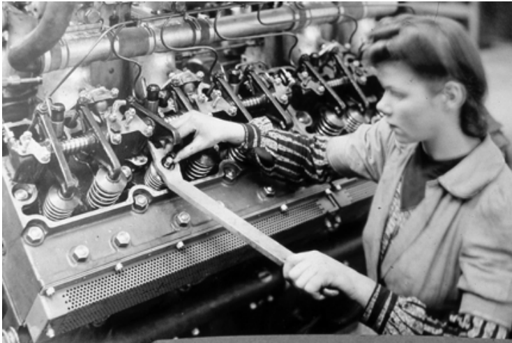
Paxman Girl assembling one of the 3,565 engines built to drive large tank and vehicle landing craft at D-Day
